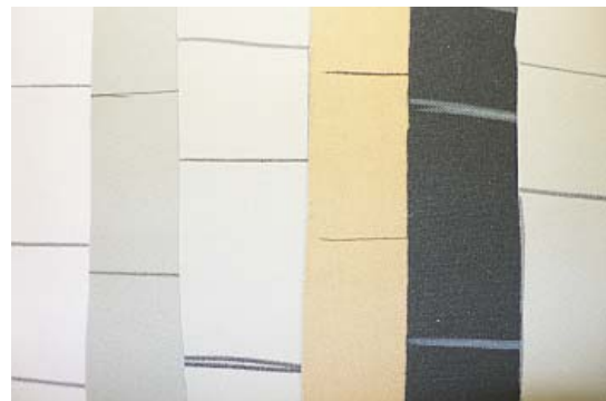
Application example: Detection of line markings on foam foil webs
