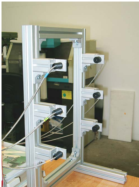
Arrangement of the SI-JET2-CON3 measuring system with 3-fold front-end on the transmitter and receiver side
