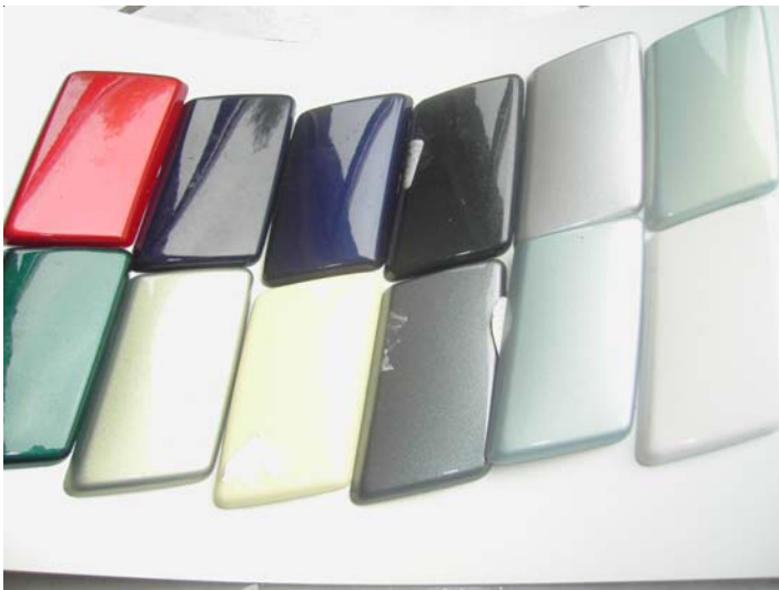
Application example: Color detection of lacquered plastic parts für car bumpers
