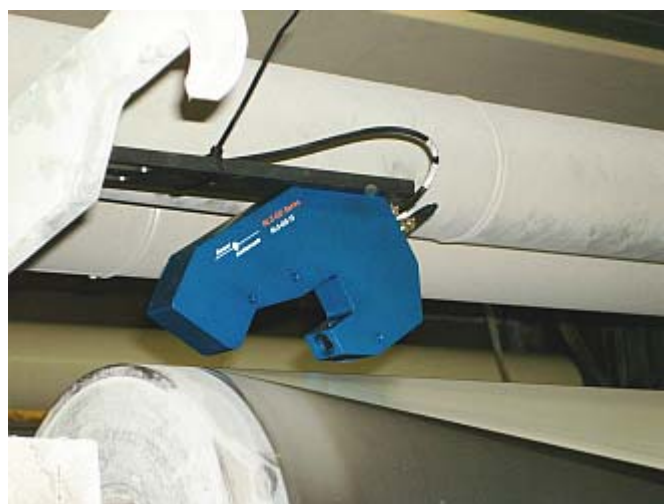
RLS-GD-15 monitoring the gloss degree of a paper web
