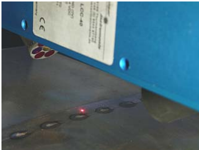
LCC-40 in the process of welding seam detection
