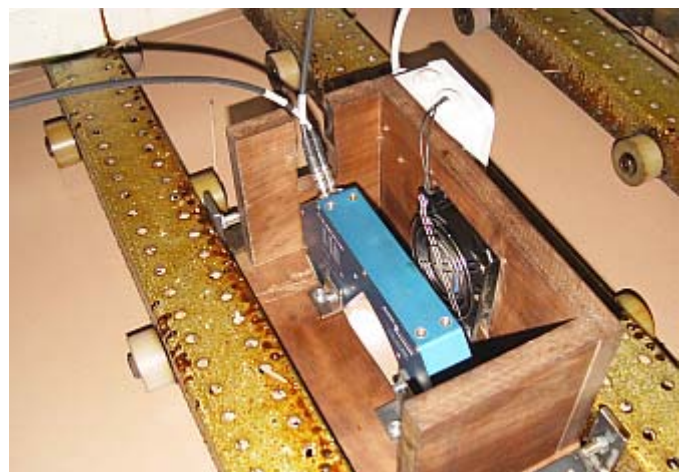
RLS-GD-60-HP with mounting facility, in the process of monitoring the back side of laminate flooring
