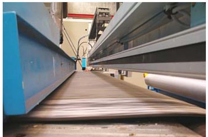
Online gloss measurement in PVC floor covering production in traversing operation
