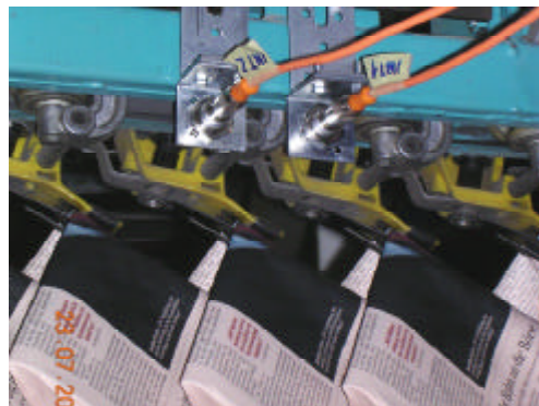
Picture 8 Counting of number of folds of paper filter elements (LCC-CON1)
